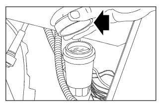
Refer to the Maintenance Schedule to determine how often to check the fluid level in the clutch master cylinder reservoir and for the proper fluid. See *Recommended Fluids and Lubricants on page 6-11*.
